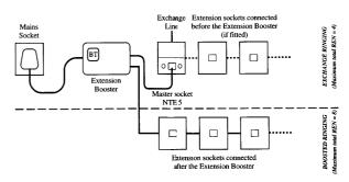
It does not matter how many sockets are connected either before or after the extension booster. It is only the REN of the equipment connected to the sockets that matters. Sockets with no equipment connected can be ignored when calculating the total REN.
